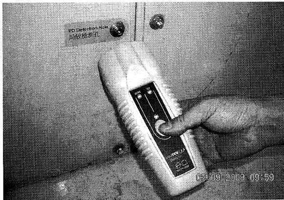
Figure 4 PD Detected on Cable Termination by Portable PD Detector
