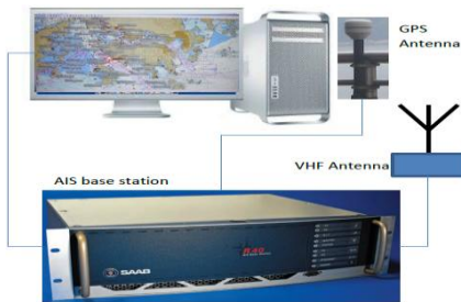
Fig. 1 - Configuration of the AIS
