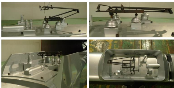
Fig. 5 – Guiding Cover of Pantograph (Simulated on Train Model)
