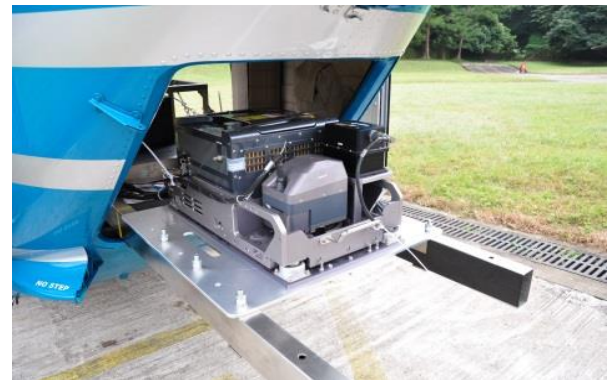
Fig. 3 – LiDAR Scanning Equipment Attached to the Helicopter
