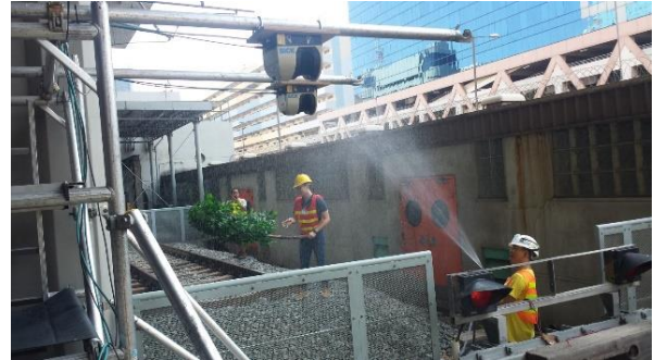
Fig. 3 – Fallen Tree Sample was detected by the LASER Detection Setup under Simulated Rains
