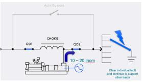
Fig. 13 - Fault located at Load Side in D-UPS
