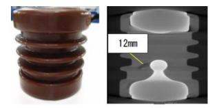
Fig. 30 - VCB Supporter and its X-Ray Image
