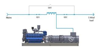
Fig. 2 - Single Line Diagram of D-UPS in Conditioning Mode
