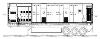
Fig. 9 - Sectional View of a BESS Container
