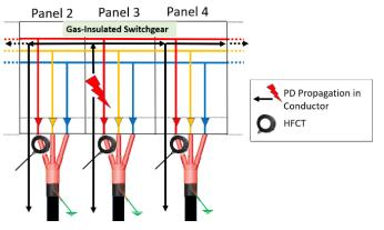
Fig. 25 - Illustration on where the PD was Located
