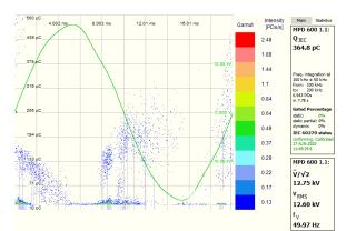
Fig. 29 - PD Result at Rated Voltage
