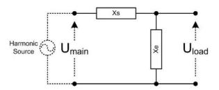
Fig. 8 - Equivalent Circuit Diagram of Voltage Harmonics in D-UPS
