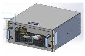
Fig. 5 - 3D Model of BMS Control Box
