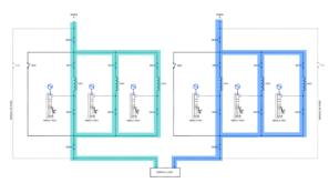
Fig. 21 - D-UPS in Parallel Arrangement (2N)
