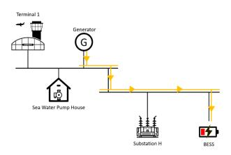
Fig. 11 - Power Flow under Green Loader Operation
