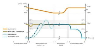
Fig. 3 - Transition of D-UPS to/from Independent Mode
