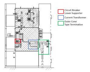
Fig. 26 - Suspected Components with PD Defect
