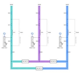
Fig. 20 - D-UPS in Distribution Redundant (N+1)
