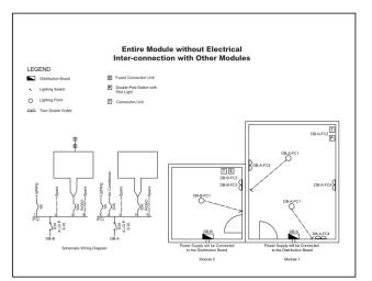
Fig. 6 - Typical Diagram of the Entire Module without Electrical Inter-connection with Other Modules
