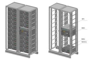
Fig. 4 - 3D Model of Battery Racks and Modules
