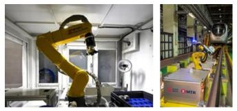
Fig. 6a - The Intelligent Relay Testing System (Left) Fig. 6b - Underframe Inspection Robot (Right)
