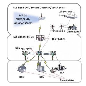
Fig. 1 - A Multi-layered Conceptual Model of the Smart Grid's Architecture
