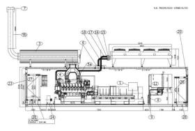
Fig. 23 - D-UPS Installation inside Container
