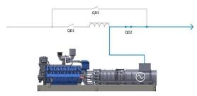
Fig. 4 - Single Line Diagram of D-UPS in Independent Mode
