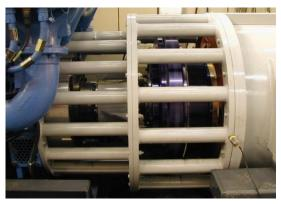
Fig. 15 - Maintenance Free Electromagnetic Clutch in mtu Kinetic PowerPack
