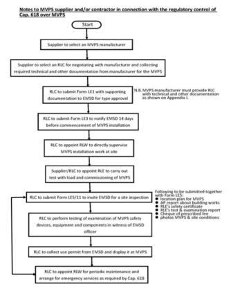
Fig. 8 - Regulatory Control of Cap. 618
