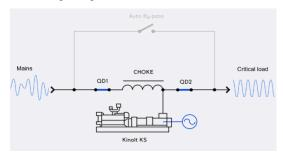
Fig. 5 - Input and Output Voltage Waveform of D-UPS in Conditioning Mode
