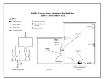
Fig. 7 - Typical Diagram of Cable Connections between the Modules at the Termination Box
