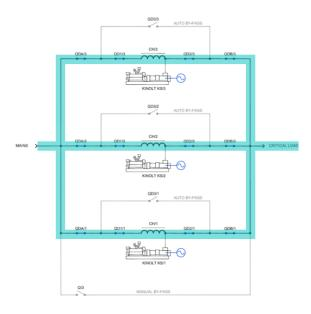
Fig. 17 - D-UPS in Parallel Arrangement (N)
