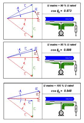
Fig. 7 - Vector Diagrams of Power Flow in D-UPS Unit
