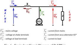
Fig. 6 - Equivalent Circuit Diagram of D-UPS in Conditioning Mode
