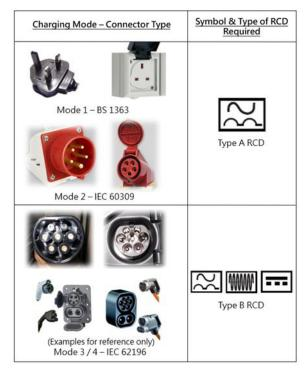
Fig. 5 - RCD Requirement for EVSE
