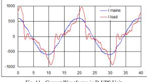
Fig. 11 - Current Waveforms in D-UPS Unit
