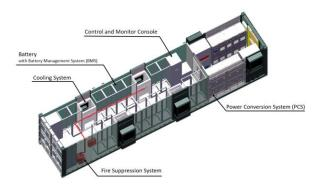
Fig. 3 - 3D Layout of BESS Container
