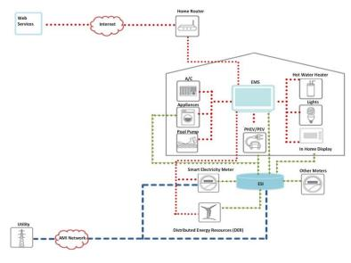
Fig. 2 - An Overview of a Smart Home's Architecture, Internal and External Environments
