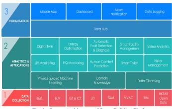
Fig. 1 - System Architecture of Smart Building Platform
