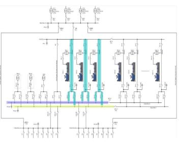
Fig. 19 - D-UPS in Parallel Arrangement with Dual Bus (N+1)
