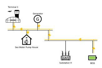
Fig. 10 - Power Flow under Emergency Backup Operation
