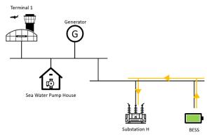
Fig. 12 - Power Flow under Peak Shaving Operation
