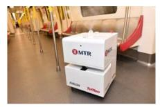
Fig. 7a - Vapourized Hydrogen Peroxide Robot
