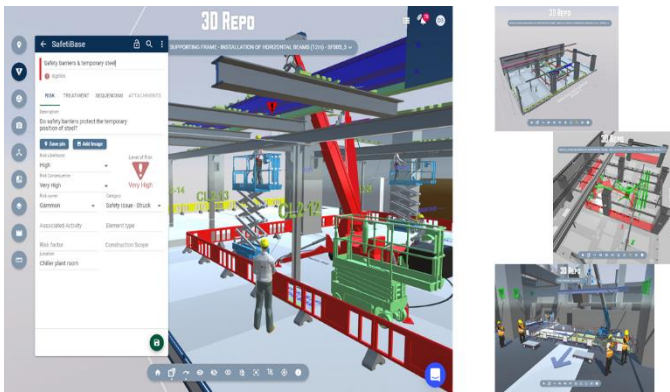
Fig. 21 - An Example using 3D Repo for Method Statement Planning to Ensure Workers Location in a Complicated Geometry and Operation of Works
