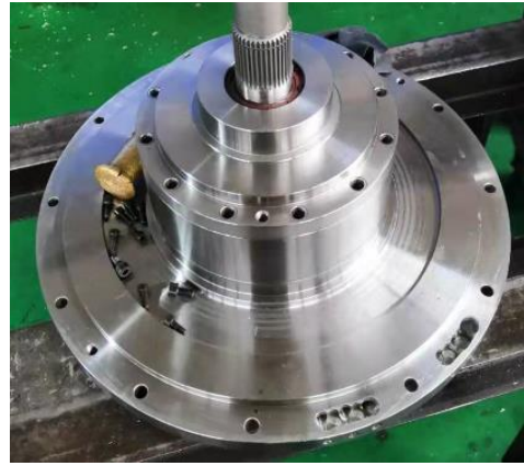
Fig. 4 - The First Stage Planetary Gearbox
