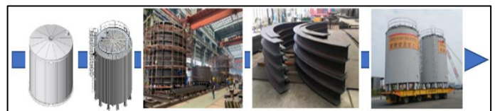
Fig. 31 – An Example of a Thermal Tank adopting DfMA Approach from BIM to Final Product
