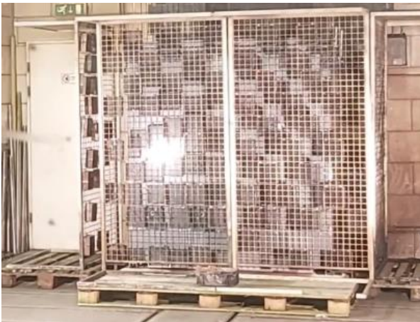
Fig. 5 - Assembly Enclosed in Cotton Indicators and Prepared for Internal Arc Fault Test
