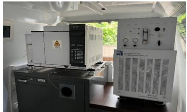
Fig. 7 - PFT Leak Location System
