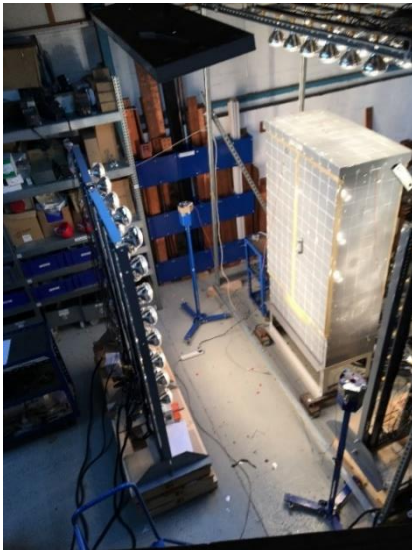
Fig. 4 - Outdoor Assembly Undergoing Temperature Rise Tests with Simulated Solar Effects
