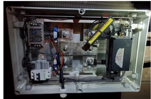
Fig. 5 - LoRa Leakage Current Sensor
