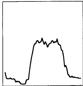
Figure 5 Load Profile of A Distribution Transformer Supplying Industrial Load
