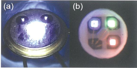
Figure 2 Laser-micromachined LED Chips
