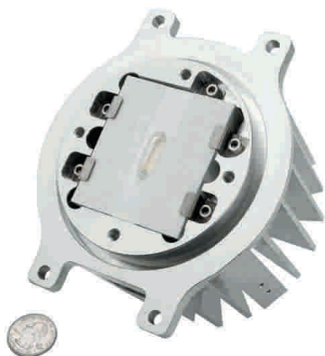
Figure 7 Sealed Quartz Bulb (the Middle Glass Tube) Immersed into the Puck to Form LEP’s Source.
