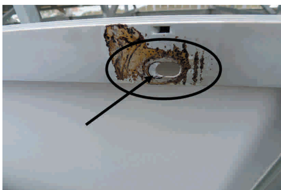
Figure 12 Corrosion Around the Mounting Hole of the Aluminium Frame of PV Panel
