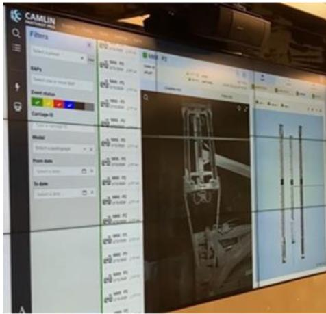
Fig. 10b – Image sent to Data Studio from Smart Train Roof and Pantograph Monitoring System
