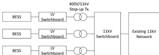
Fig. 8 - Electrical Block Diagram of BESS System
