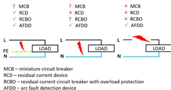
Fig. 11 - Characteristics of Different Protective Devices under Arc Faults
