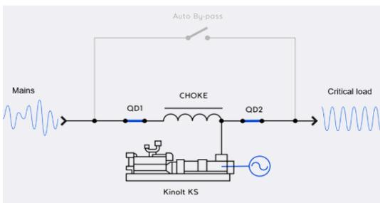
Fig. 5 - Input and Output Voltage Waveform of D-UPS in Conditioning Mode
