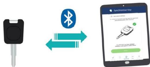
Fig. 17 - Pairing of Key to Tablet App through Bluetooth
