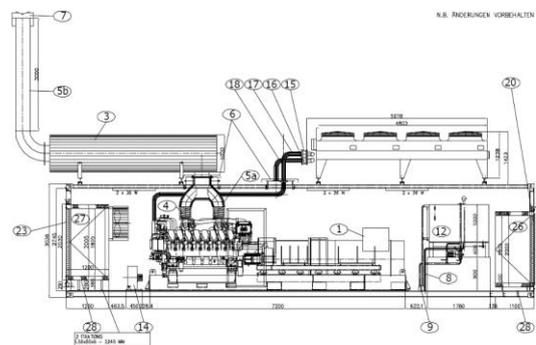
Fig. 23 - D-UPS Installation inside Container
