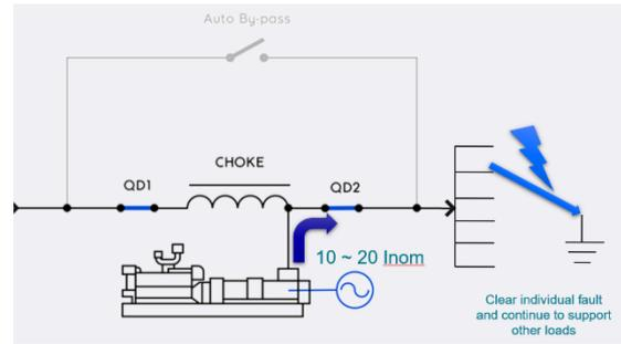
Fig. 13 - Fault located at Load Side in D-UPS
