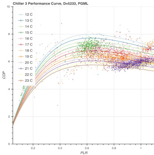
Fig. 4 - Physics-guided Machine Learning for Chiller Model Development (with Predictability outside the Range of Available Data)
