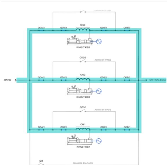
Fig. 18 - D-UPS in Parallel Arrangement (N+1)
