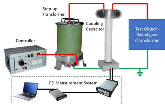
Fig. 27 - Offline HVAC PD Test according to IEC60270
