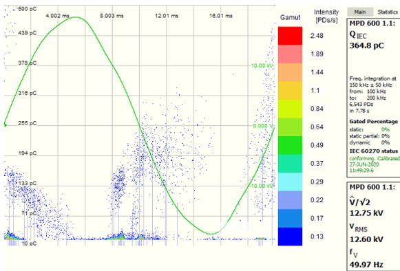
Fig. 29 - PD Result at Rated Voltage
