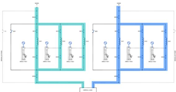
Fig. 21 - D-UPS in Parallel Arrangement (2N)
