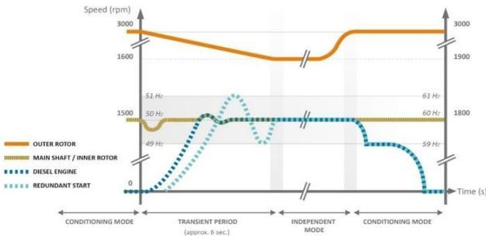
Fig. 3 - Transition of D-UPS to/from Independent Mode
