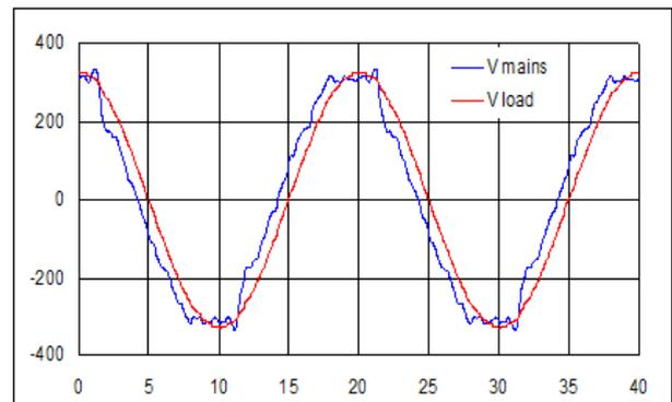
Fig. 9 - Voltage Waveforms in D-UPS Unit
