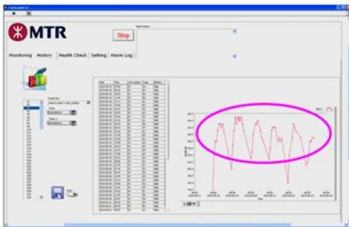
Fig. 8b - RFID Real-time Temperature Monitoring System Displayed in Control Centre Equipment
