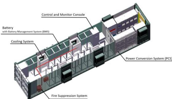
Fig. 3 - 3D Layout of BESS Container
