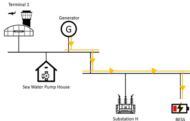
Fig. 11 - Power Flow under Green Loader Operation
