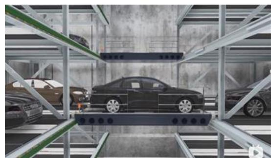
Fig. 6 - Vertical Lifting Horizontal Sliding (VLHS)
