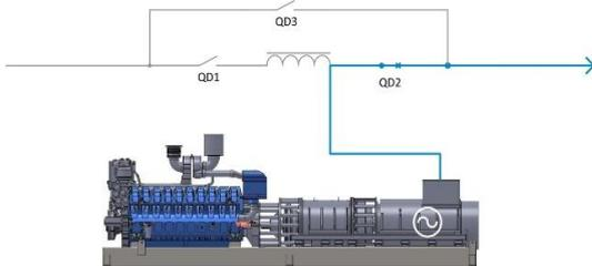
Fig. 4 - Single Line Diagram of D-UPS in Independent Mode
