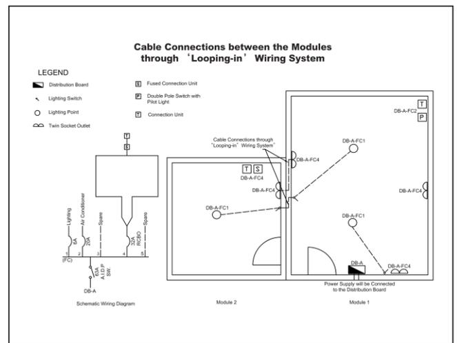
Fig. 8 - Typical Diagram of Cable Connections between the Modules through “Looping-in” Wiring System
