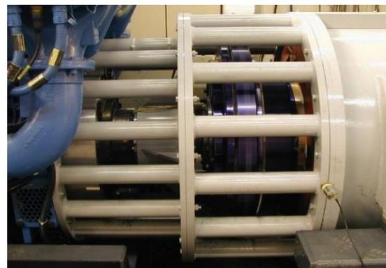
Fig. 15 - Maintenance Free Electromagnetic Clutch in *mtu Kinetic PowerPack*
