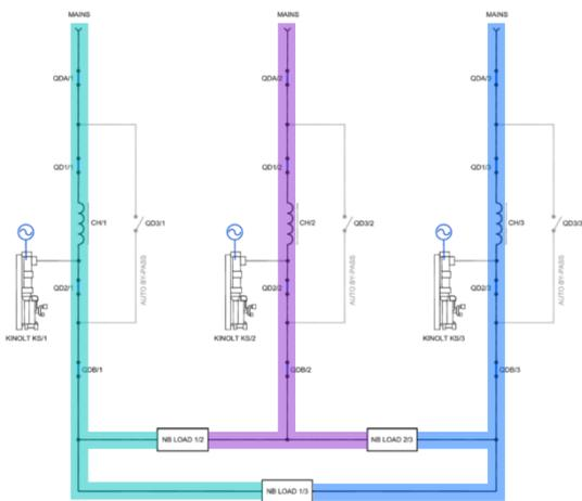
Fig. 20 - D-UPS in Distribution Redundant (N+1)
