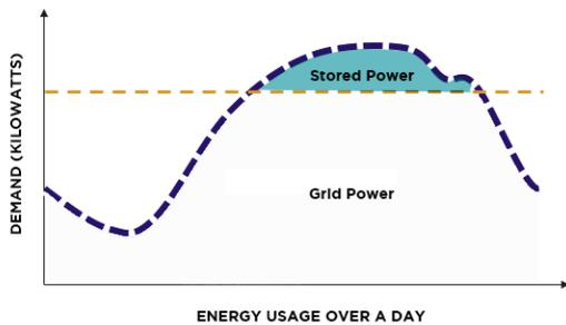
Fig. 13 - Power Peak Shaved by Stored Energy of BESS
