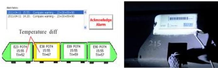
Fig. 8a - RFID Real-time Temperature Monitoring System of Train Equipment
