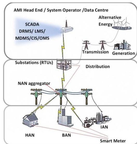
Fig. 1 - A Multi-layered Conceptual Model of the Smart Grid's Architecture
