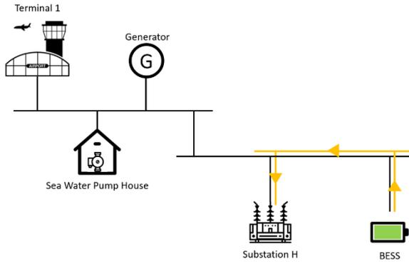
Fig. 12 - Power Flow under Peak Shaving Operation
