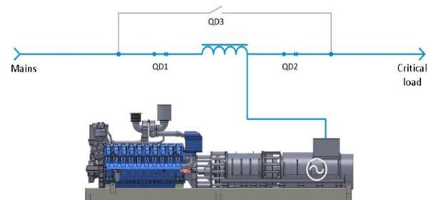
Fig. 2 - Single Line Diagram of D-UPS in Conditioning Mode
