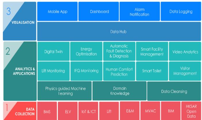
Fig. 1 - System Architecture of Smart Building Platform
