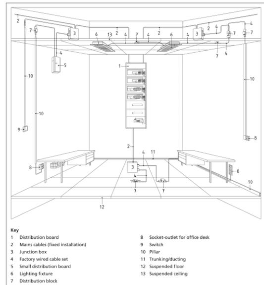
Fig. 10 - Diagrammatic Presentation of a Typical Prefabricated Wiring System
