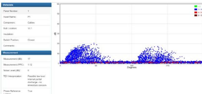
Fig. 4 - PRPD Diagram of TEV Measurement
