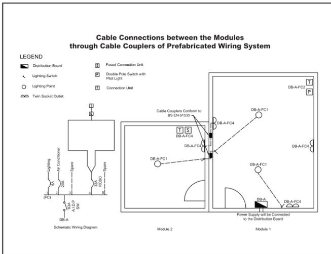
Fig. 9 - Typical Diagram of Cable Connections between the Modules through Cable Couplers of Prefabricated Wiring System
