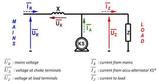
Fig. 6 - Equivalent Circuit Diagram of D-UPS in Conditioning Mode
