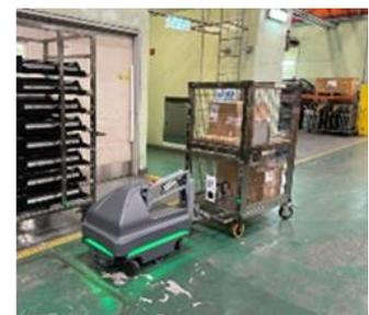
Fig. 5b - Lift-type SLAM-based AGV (Right)
