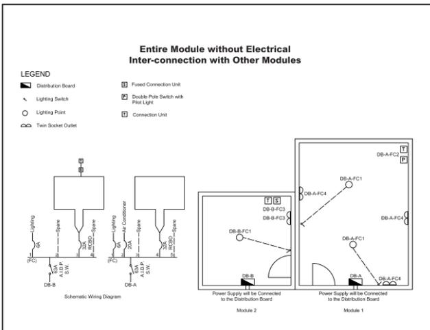
Fig. 6 - Typical Diagram of the Entire Module without Electrical Inter-connection with Other Modules
