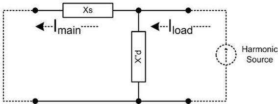
Fig. 10 - Equivalent Circuit Diagram of Current Harmonics in D-UPS
