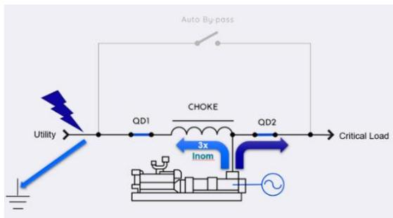
Fig. 12 - Fault located at Utility in D-UPS System
