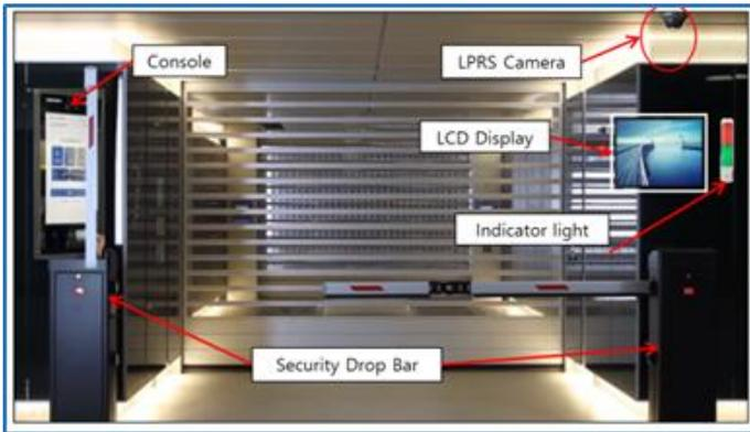
Fig. 8a - Example of Kiosk and Monitoring Devices Outside at the Transfer Cabin
