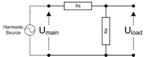
Fig. 8 - Equivalent Circuit Diagram of Voltage Harmonics in D-UPS
