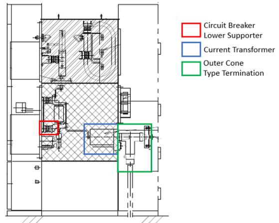
Fig. 26 - Suspected Components with PD Defect
