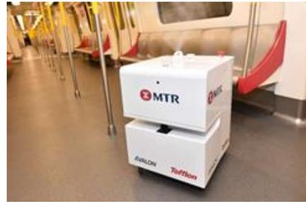
Fig. 7a - Vapourized Hydrogen Peroxide Robot
