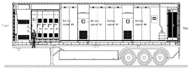
Fig. 9 - Sectional View of a BESS Container
