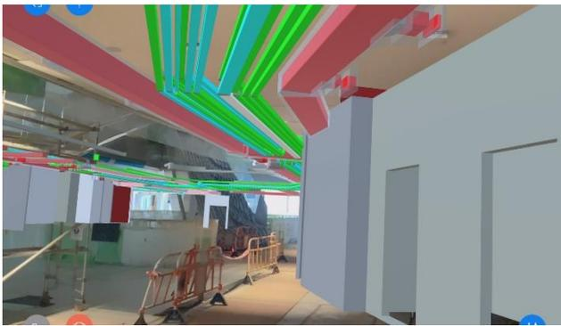
Fig. 18 - Snapshot on Tablet Screen for Superimposed BIM into Actual Site
