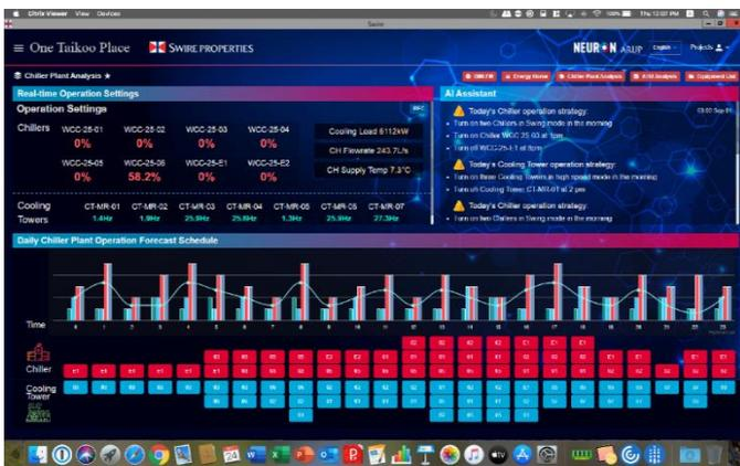
Fig. 21 - Snapshot for AI & ML Advice on Chiller Plant Operation after Energy Optimization
