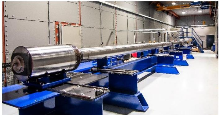
Fig. 3 - The Two-stage Light Gas Gun used to Accelerate Projectiles Up to 6.5 km to Achieve Projectile Fusion (©First Light Fusion Limited, 2021)
