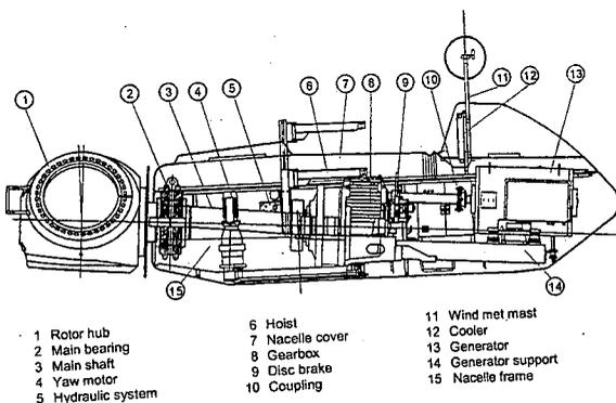
Technical particulars of the N50/800kW wind turbine are as follows:
