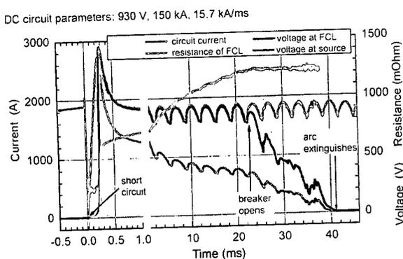
These severe DC test experiments clearly show the high potential and the technical feasibility of SFCL.
