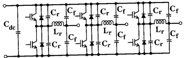
Resonant pole inverter is to use  $C_r$  and  $L_r$  to resonate the voltage across the switching devices to zero when they are turning on and off. Each inverter leg has a resonant circuit formed by  $L_r$  and  $C_r$ . Because the condition of the zero-voltage resonance is limited by the load condition, an improved variable frequency modulation has been developed and used in industrial drives [27].
