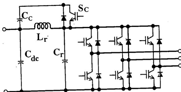
Resonant DC link inverter is basically to resonate the DC link voltage using resonant inductor  $L_r$  and resonant capacitor  $C_r$  such that when the inverter transistor is to switch under zero resonant voltage to eliminate the switching loss of the inverter and EMI. Because the resonant voltage is high, around twice of the input voltage, a clamping circuit is usually used that is formed by  $C_c$  and  $S_c$  so that the maximum resonant voltage is controlled to 1.3 of the DC input voltage.
