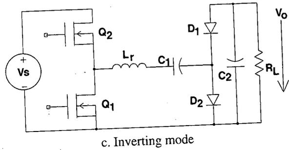
Figure 2 A High Power Density Switched-Capacitor Converter
