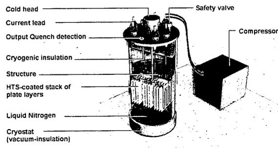
The limited current  $I_{lim}$  is mainly determined by the thickness of a metallic shunt layer and can be adjusted to about  $0,1 - 5 I_n$  as long as the protection against hot-spots is maintained.
