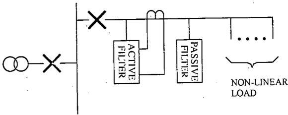
In order to ascertain the effectiveness of the hybrid filter, an installation (comprising a 430A passive filter and a 120A active filter) in which the connected feeder circuit is for office supply loads with a rated current of 800A rising main has been studied. Examinations of the filter performance in following various test scenarios are carried out :-
