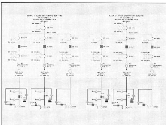
The 500kV Open Type Switchyard facilities are supplied by Mitsubishi Electric Corporation. Electricity output from each power block is connected to an individual single 525kV bus group which is then transported to EGAT's existing Ratchaburi 3 Substation via an individual group of 500kV overhead line.
