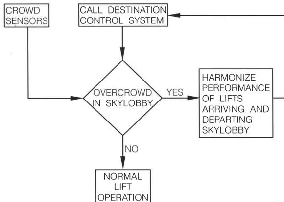
**Figure 8 Double Deck Lift Traffic Concept**
