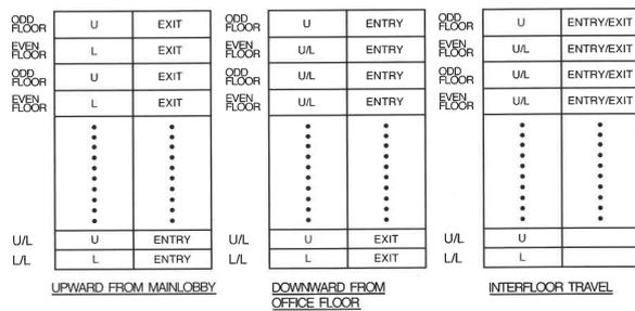
The compact size of the building core of ICC is attributed to the adoption of double deck local passenger lifts and shuttle lifts.
